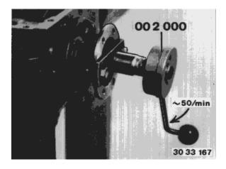
Establish friction torque level of new differential housing bearings. The axial preload force of the differential housing bearing (4000 N) can be determined from the friction torque, refer to Technical Data.
