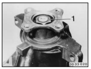
Punch mark both bearing caps. Unscrew and remove both bearing caps.
