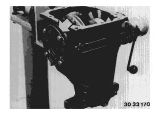
refer to Technical Data, a thicker shim must be installed on the crown gear side and the measurement must be repeated.
