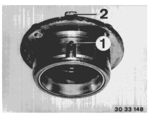
Press outer bearing race out with special tool 33 1 350 / 351.
