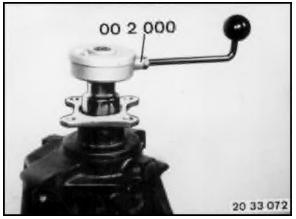
Measure friction torque, refer to Technical Data, with special tool 00 2 000 and suitable socket.
