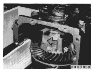
To check the tooth contact pattern, coat the crown wheel teeth with printer's ink, turn in both directions several times and stop crown wheel suddenly with a piece of hard wood.
