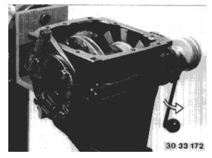
To make it easier to establish the correct shim thickness, the gap between shim and transmission case can be measured with a feeler gauge and added to the thickness of shim used.
