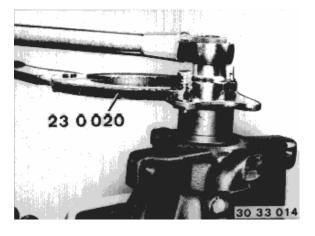
Tighten input flange with the collar nut in steps, measuring the friction torque after each step.
