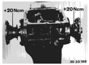
Install an output flange on the side opposite of the crown wheel. Using a bracket with welded nut (in-house manufacture) and special tool 00 2 000, establish level of friction torque.
